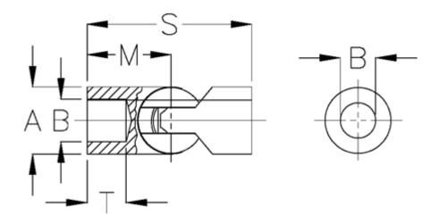
A = 110 B H7 = 75 M = 160.0 Max torque (Nm) = 1370 s = 320 T = 85
